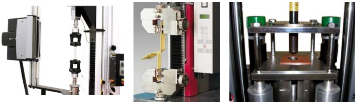
Fig. 14: machines for tensile, tear resistance and puncture impact tests (left to right)
